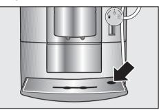
Replace the drip tray cover. Be sure the outer hole is located under the cappuccinatore.
